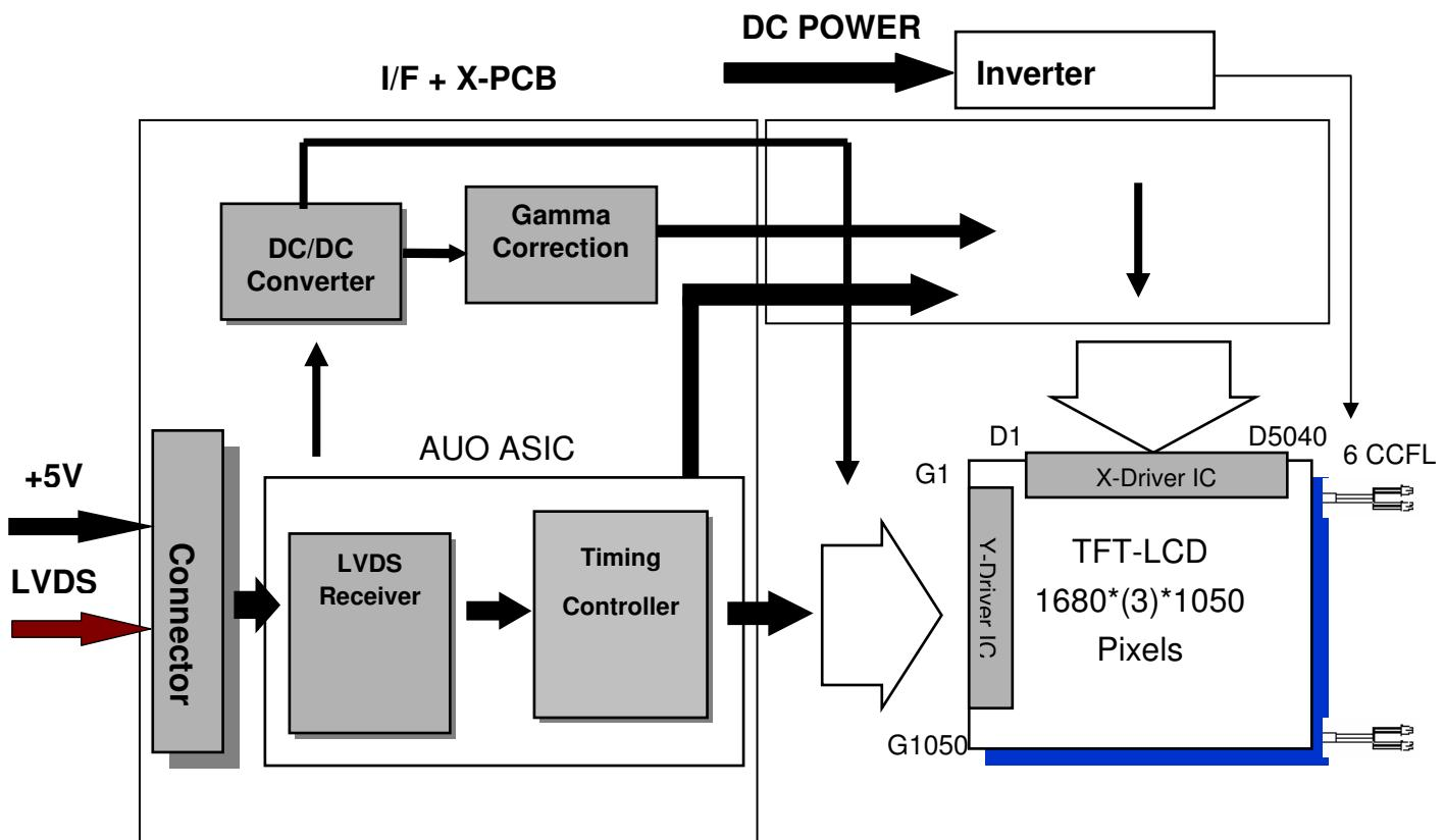
LVDS Connector: JAE (FI-XB30SRL-HF11) or equivalent.
